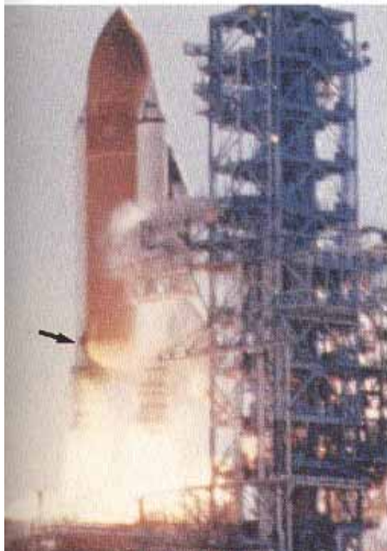
Image 7: Smoke Puffs from 0.836 s continued to 2.500 seconds, occurring about 4 times a second. smoke source shown in computer generated drawing. (13)
