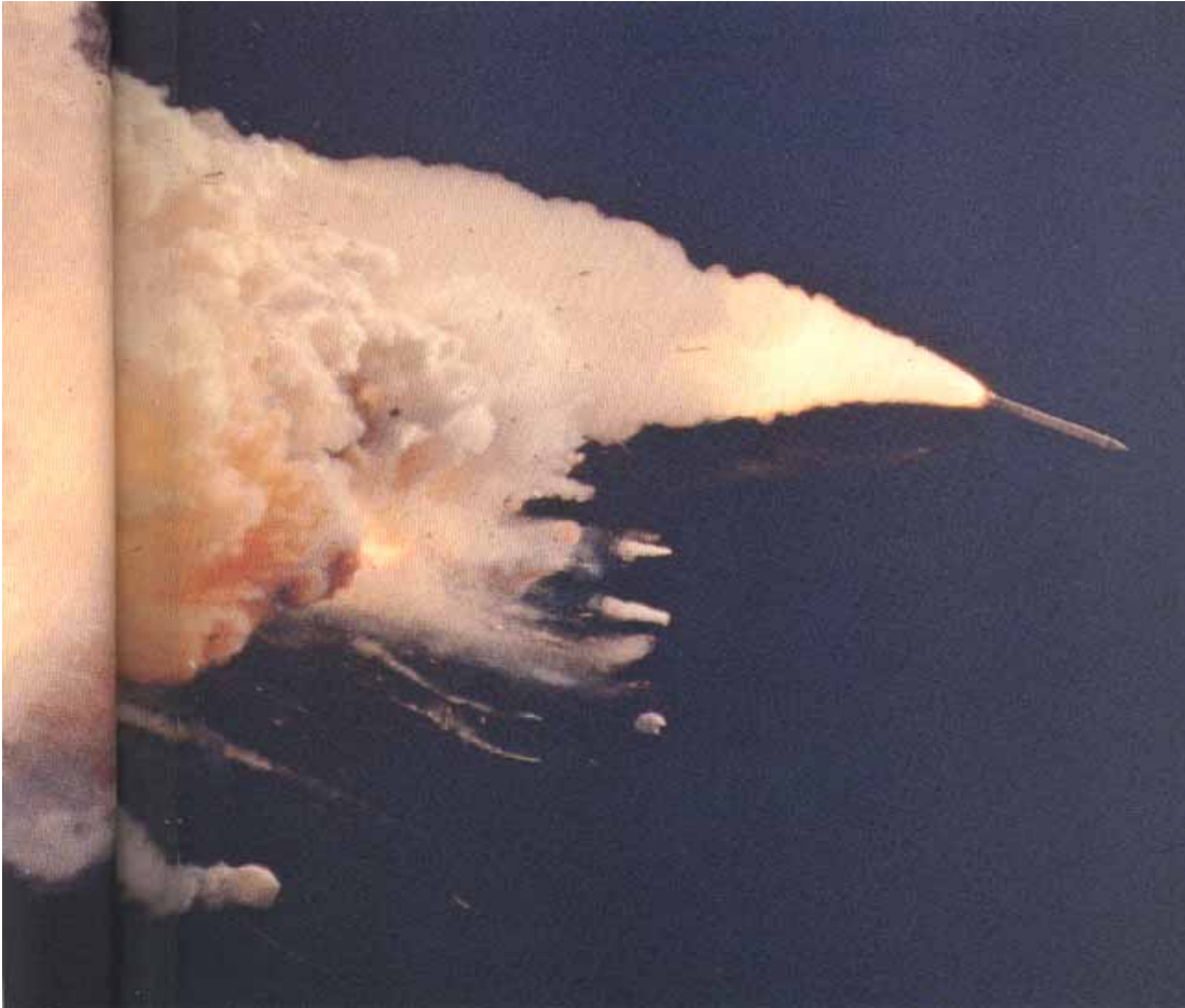
Image 11: Explosion at 76 s in flight, left SRB soars away, still thrusting. (17)
