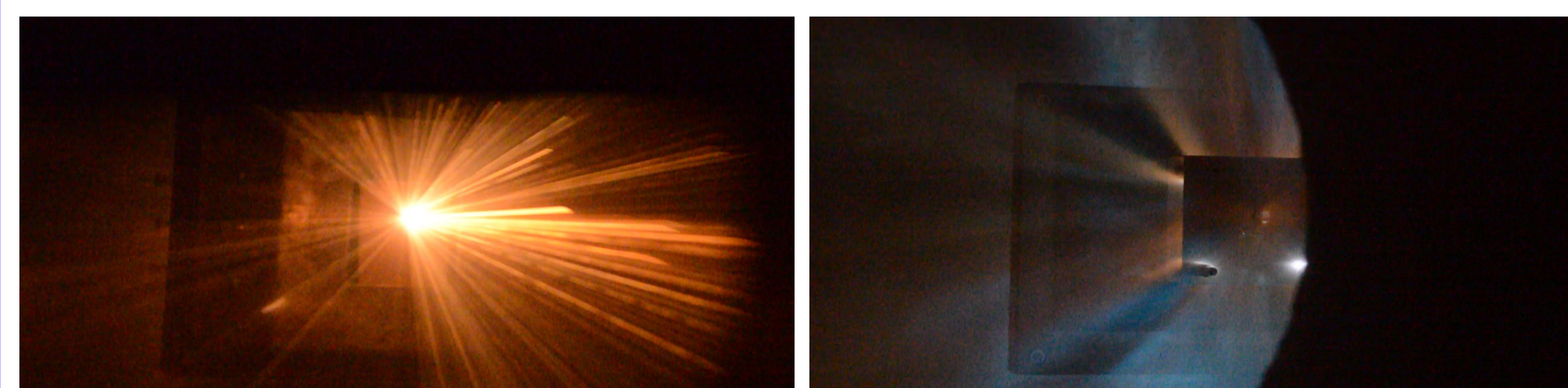
Figure 5: Extracted images from video footage: Left: 1 mm diameter stainless steel projectile impacting sandstone at 5.16 kms -1 (shot ID G051012#3). Right: Solid sabot projectile impacting Aluminium plates at 5.38 kms -1 (shot ID G141212#2).
