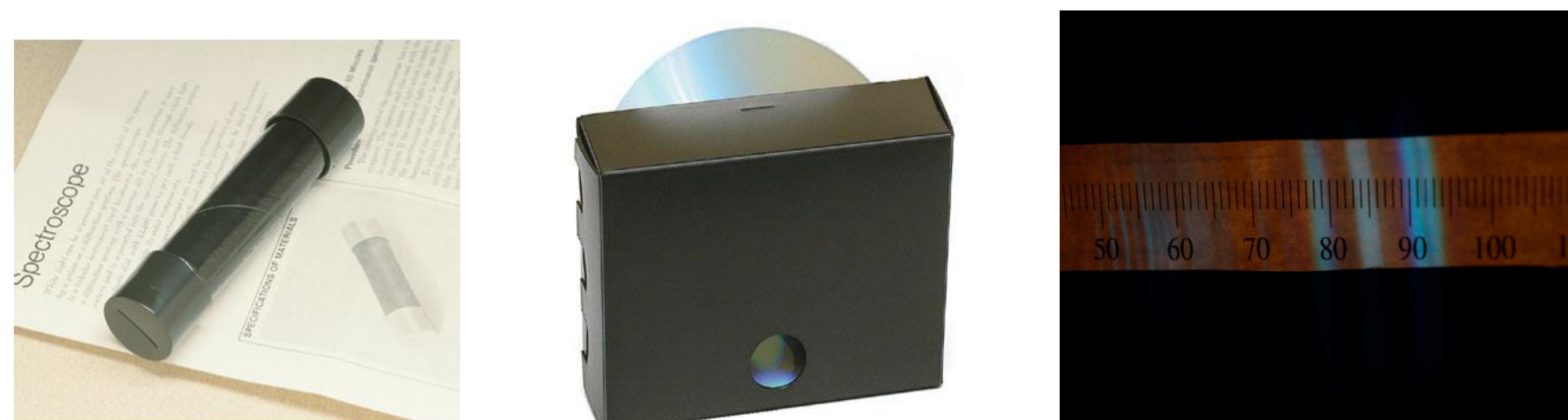
Figure 2: Some low-cost spectroscopes which were tested and did not work, as well as an early attempt to photograph a spectrum of a Cadmium emission lamp.
