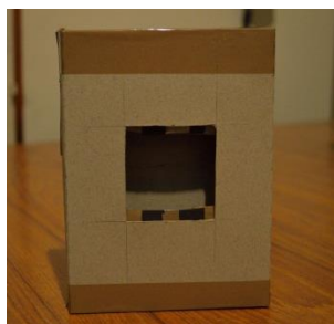
Figure 19: First attempt of self-build spectroscope
