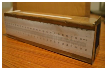
Figure 20: Self-build spectroscope with scale
