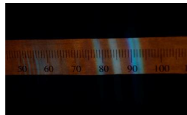
Figure 21: Attempt of photographing a Cadmium emission lamp spectrum
